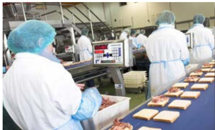
**The Takeaway LineMaster® workstations employed across Greencore's sites are ideal for fast, accurate portioning of food items. As with all MARCO's scales, the LineMaster® includes a traffic light weighing system, proven to increase packing speed and accuracy.**
