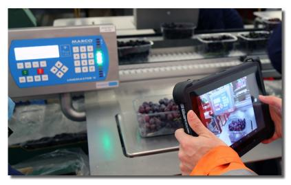
The labeller system has a printer fitted for direct on-line printing. The labeller heads are synchronised with the pack and the conveyor, with the capability of linear speeds up to 40 metres per minute. This ensures accurate label positioning on the packs within  $\pm 0.2$ mm.
